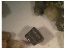
Photo 50 – chromite – dissolution pattern – 1.5mm
