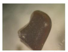
Photo 37 – SG-87 – Altered silicate (serpentine?) – 1.4mm – All sides frosted, etc
