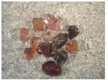
Photo 33 – garnets with zero pickup, ~no iron
