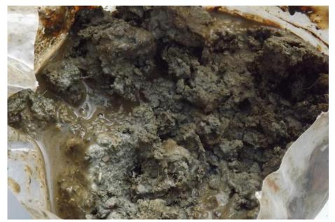
Photos D & E: From Traverse 4, Sample 3 – Wet Clay/Till
