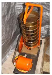
2 -Tyler motorized portable sieve shaker
