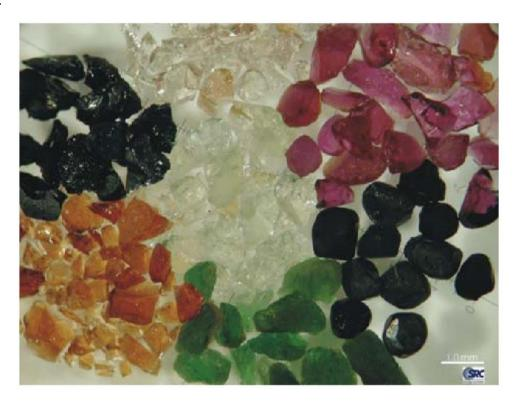
Photo K, "Kimberlite Indicator Minerals. From top left-clockwise: picroilmenite (Mg-rich ilmenite); eclogitic Fe-Mg-Ca almandine G3 garnets; peridotitic chrome pyrope G9/G10 garnets; chromites; chrome diopsides; Ti-Cr-Mg pyrope G1/G2 garnets; and olivines in the centre" (Quirt, 2004, p 2).
