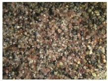
Photo 119 – unpicked cons from GoldCube – Fine-to-medium sand fraction
