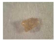
Photo 40 – SD-7 – Silicate (Epidote) – 0.8mm
