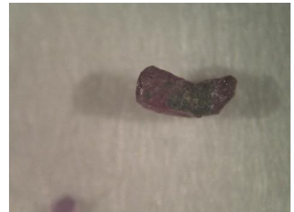
C - (same as B & D) – showing frosted surface & attached kimberlite
