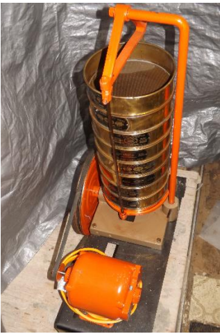
2 - Tyler motorized portable sieve shaker
