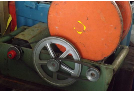
4 - Variable speed industrial tumbler
