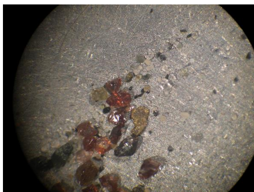
5 - Gold grain 1 \times 0.5 \times 0.2 mm from -35 fraction with other KIMs, TP
