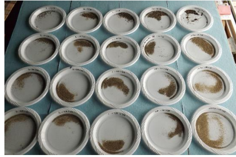
1a - Panned and dried concentrates from sluice efficiency test ready to pick for KIMs under microscope
