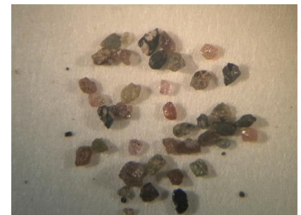
Photo 21 – Trench – almost inert – probable KIMs
