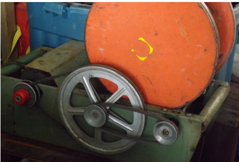
4 - Variable speed industrial tumbler
