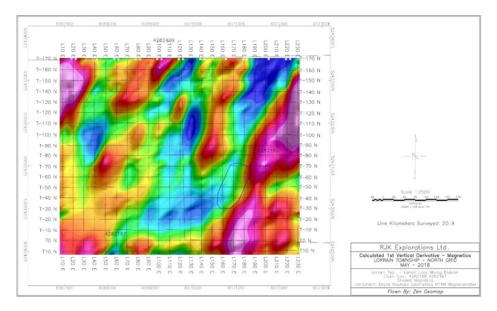
Figure 12: Calculated 1st Derivative – Magnetics, Cedar Pond
