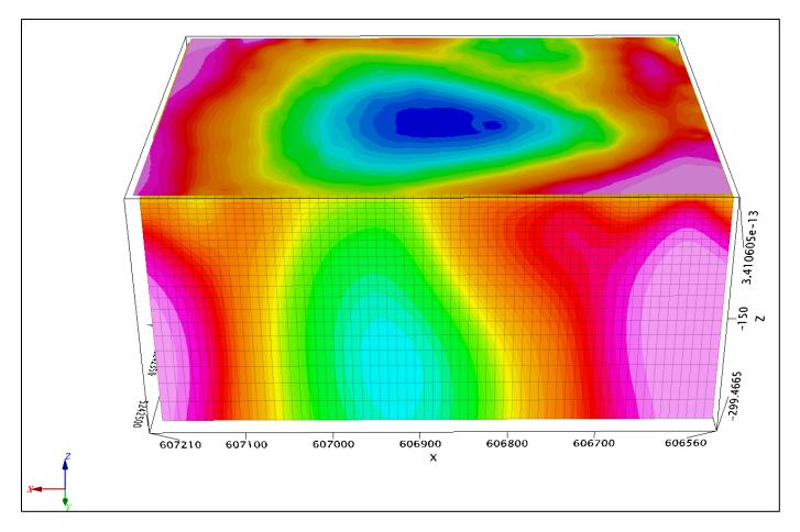
Figure 5: 3D Voxel looking South at inclination 29 degrees. Paradis Pond
